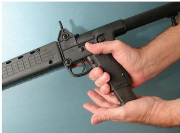
and outside the trigger guard. Insert the loaded magazine into the grip until it is locked in place. Check to assure that the magazine is secure. Pull the bolt back and release. If the bolt is already back, pull back a short distance rotate right and allow the bolt to carry fully forward. This strips a round from the magazine and seats it in the barrel chamber.
