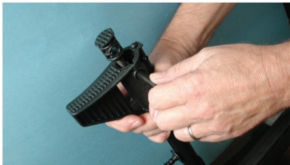
**We strongly discourage from unscrewing the stock collar, barrel or removing the front sight. These parts are assembled by special tools and compounds.**
