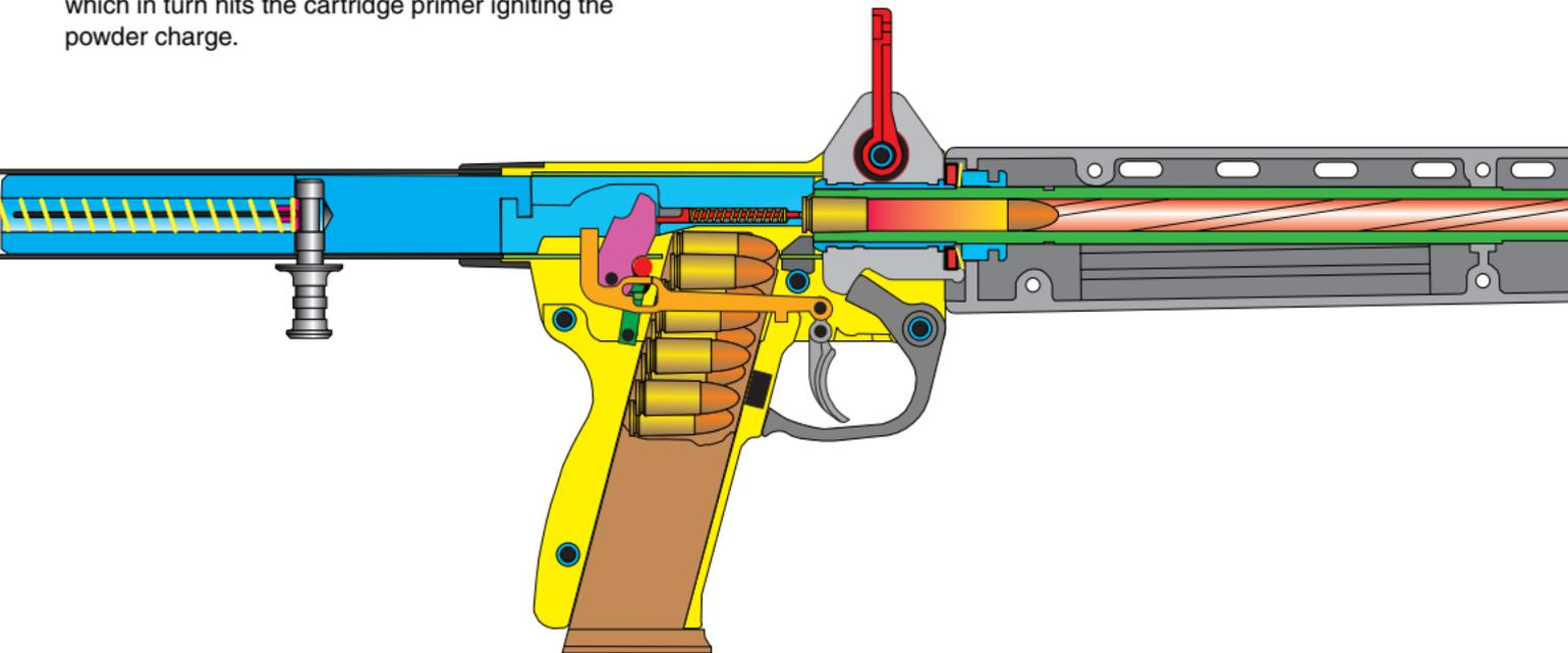
After about 3/16 (5 mm) of bolt travel (or .0013 seconds) the bullet exits the muzzle. The pressure in the barrel has now dropped to a low level.
